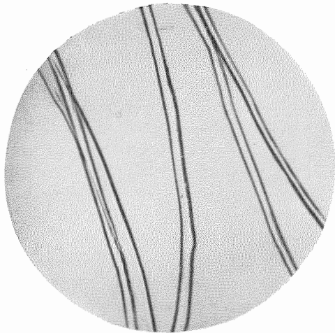
Figure 15—Insusilk C Fibres made from Mulberry Silk (Magnification 200 approximately).
