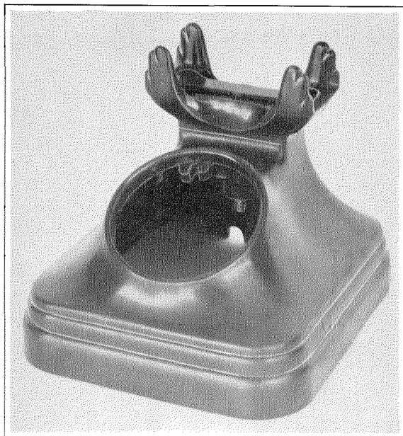
Figure 1—Subscriber Set Housing with Cradle.
